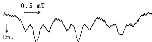
Fig. 1. CIDEP spectrum of TNA in a 2-propanol-water mixture; time delay 0.2 \mu s, gate width 0.2 \mu s.
